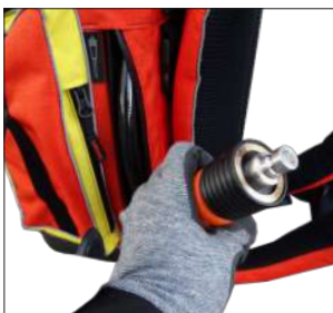
connection to a B.A.S., B.A.S. superlight or a B.A.S. optima hydraulic power unit
