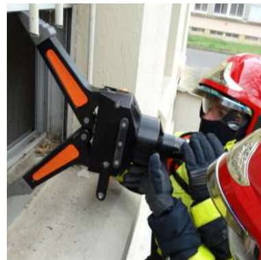
fast hydraulic spreader with controlled action
